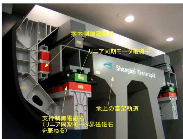
(a) Structure of electromagnetic suspension and guidance magnets and linear synchronous motor
