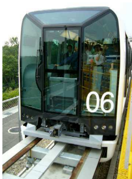
図 4 電磁吸引形磁気浮上リニア誘導モータ推進の LINIMO Fig. 4 LINIMO, a Japanese Maglev with electromagnetic suspension and linear induction drives.
