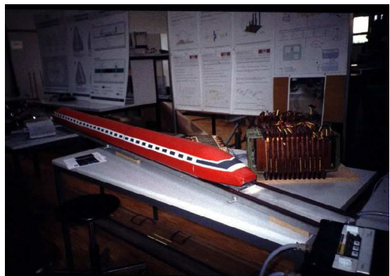
(b) Reduced vehicle model and a part of armature of a homopolar linear motor
