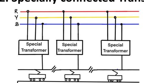
Specially connected transformers like Scott, LeBlanc, V-v tap all the three phases at each substation.
