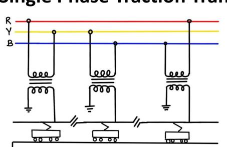
Two phases are tapped from the grid in cyclic permutation at each substation
