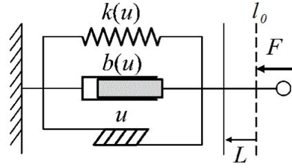
Fig. 2. Muscle viscoelastic model.
