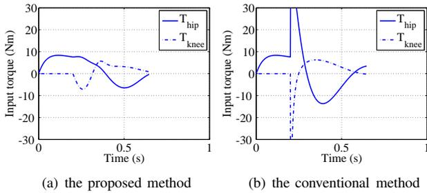
Fig. 11. Input actuator torques in the proposed and conventional methods.
