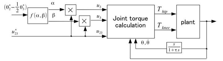
Fig. 5. Block diagram of the proposed method.  $f(\alpha, \beta)$  denotes the ratio of muscle contraction force calculated by (15) and (16).
