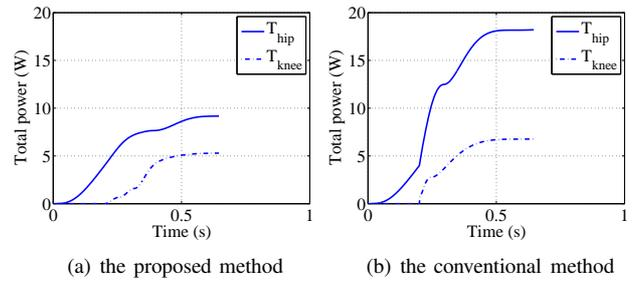
Fig. 12. Evaluation values of total energy consumption in the proposed and conventional methods.
