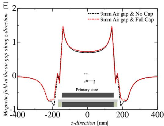
Fig. 7. Distribution of air gap flux density along z-direction
