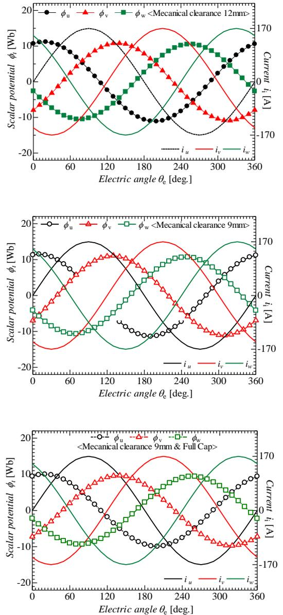
Fig. 6. Absolute value and phase relation between scalar potential and applied current in steady state in 3 models
