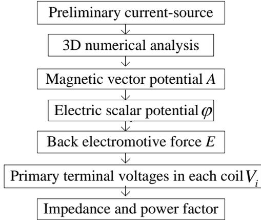
Fig. 2. Flowchart of impedance calculation
