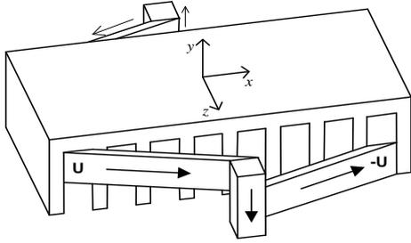
(c) Three dimensions of one U-phase coil model
