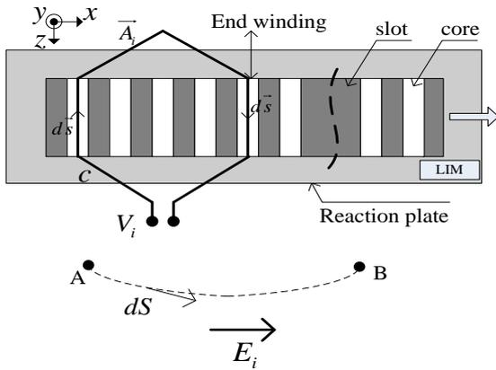
Fig. 3. Assumption of integral route in line integral of magnetic vector potential
