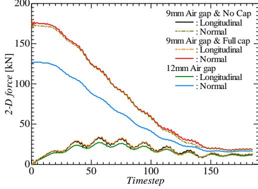
Fig. 5. 2-D force characteristics of 3 models of LIM at motor starting transient
