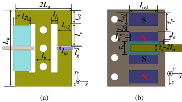
Fig. 2. Specifications of parts. (a)  $x$ - $y$  plane. (b)  $x$ - $z$  plane. (In (a), armature coils and non-magnetic material on the right side are removed for clarity.)
