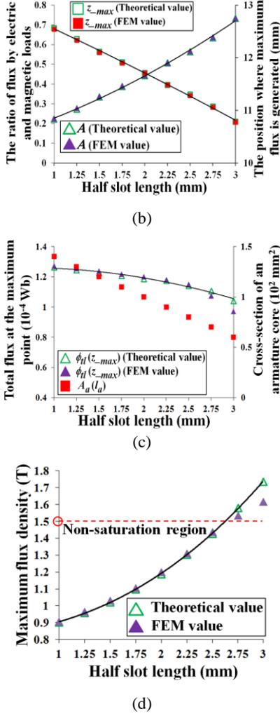
Fig. 7. Theoretical and 3D FEM results. (a)  $\phi_{ml\_max}$  and  $\phi_{el\_max}$ . (b)  $A$  and  $z_{max}$ . (c)  $\phi_H(z_{max})$  and  $A_a(I_a)$ . (d)  $B_{max}$ .
