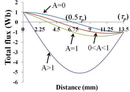
Fig. 5. Total flux distribution by the flux ratio  $A$ .
