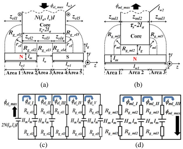
Fig. 6. Magnetic circuit models for flux calculation by electric and magnetic loads. (a) Model at  $z = 0.5\tau_p$ . (b) Model at  $z = 0$ . (c) Equivalent magnetic circuit at  $z = 0.5\tau_p$ . (d) Equivalent magnetic circuit at  $z = 0$ . (Only a half model is illustrated because of the symmetric structure.)
