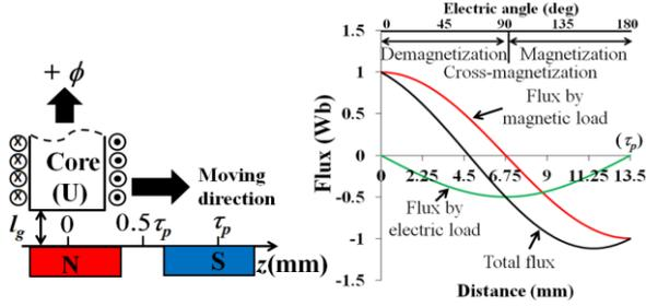
Fig. 4. Flux distribution in the armature core due to armature reaction. (The positive value on the left side represents the direction in which the flux flows into the iron core.)
