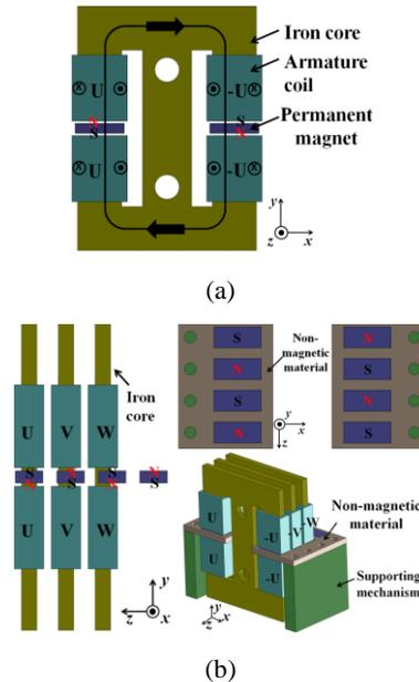
Fig. 1. The basic configuration of the three-phase unit. (a) Armature and field units. (b) Configuration along the moving direction. (In (a), black arrows denote flux flow under a no-load condition. In (b),  $-U$ ,  $-V$ , and  $-W$  are present components shifted by 180 degrees from  $U$ ,  $V$ , and  $W$ .)
