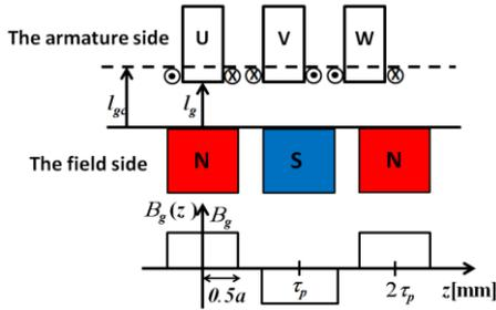
Fig. 3. Flux density distribution resulting from moving an armature unit.
