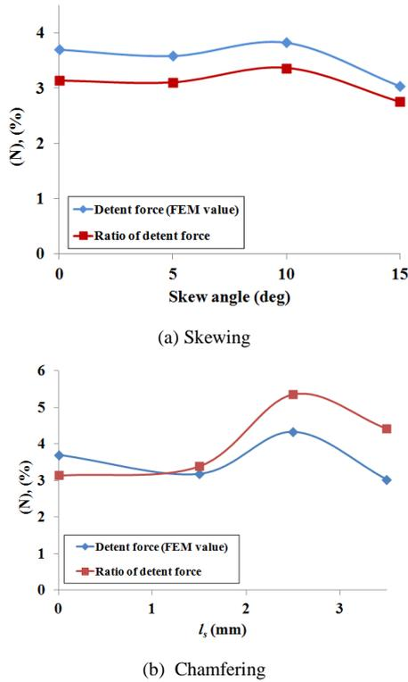
Fig. 9. Ratio of detent force to thrust based on 3-D FEM results.
