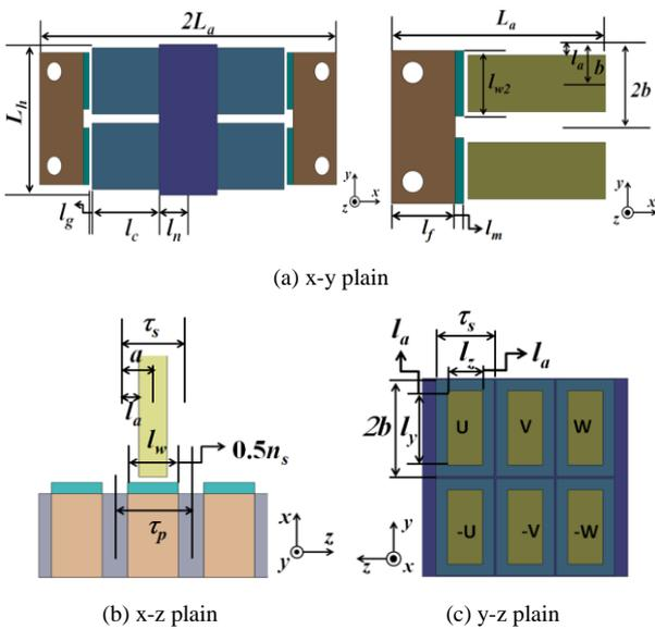
Fig. 2. Variables employed in the design (In (a) and (b), the armature coils are removed for clarity. Also, variables are labeled in the half side because of symmetric structure.).
