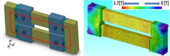
(c) A magnetic circuit (In (c), the red arrows denote flux flow; the non-magnetic material box was removed for easy understanding.)
