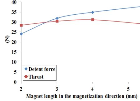
(b) Thrust and detent force based on 3-D FEM result at  $l_a=3.5$ mm
