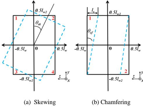
Fig. 7. Skewing and chamfering. (The dashed lines denote skewed and chamfered magnets.)
