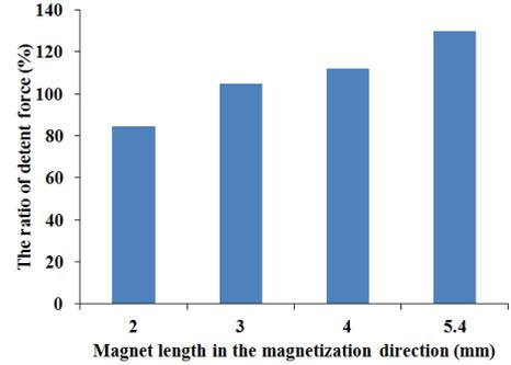
(c) Ratio of detent force to thrust based on 3-D FEM result at  $l_a=3.5$ mm
