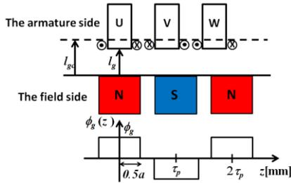
Fig. 3. Effective flux distribution resulting from moving an armature unit.
