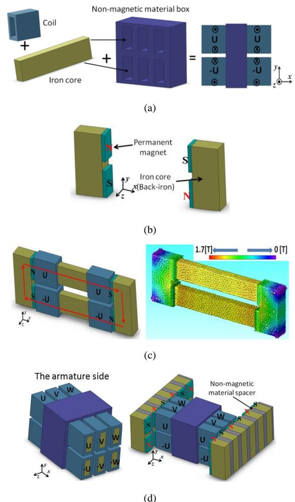
Fig. 1. Fundamental configuration of the three-phase unit. (In (c), the red arrows denote flux flow; the non-magnetic material box was removed for easy understanding.) (a) An armature unit (mover). (b) A field unit (stator). (c) A field magnetic circuit. (d) Configuration along the moving direction.
