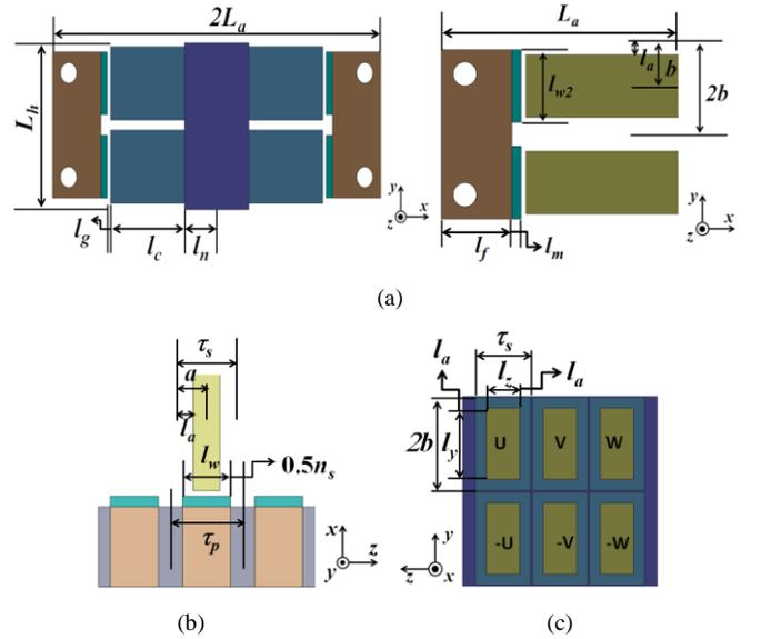
Fig. 2. Variables employed in the preliminary design (In (a) and (b), the armature coils are removed for clarity. Also, variables are labeled in the half side because of symmetric structure.). (a) x-y plain. (b) x-z plain. (c) y-z plain.
