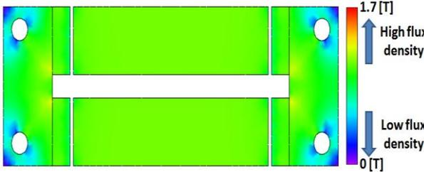
Fig. 6. Flux density distribution of the proposed model.
