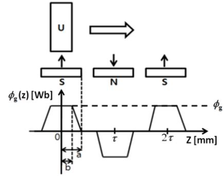
Fig. 4. The air gap flux distribution by moving an armature unit.
