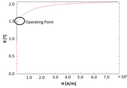
Fig. 5. B-H curve of 50JN230 (JFE Steel Corp.)
