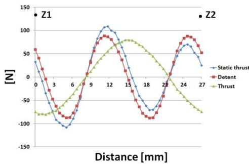
Fig. 11. Static thrust, detent force and thrust in rated region.
