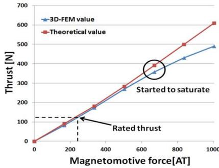
Fig. 10. Thrust-current characteristics.
