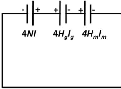
Fig. 3. Equivalent magnetic circuit considering an magnetic circuit.
