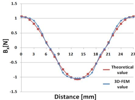
Fig. 7. The air gap flux density.
