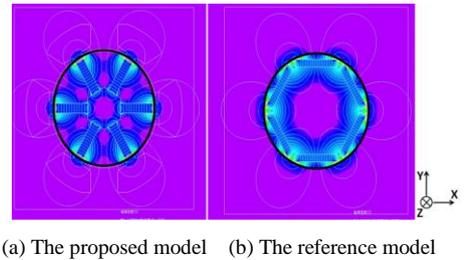
Figure 8: The flux density distribution without the armature side (The circle is an air gap section).
