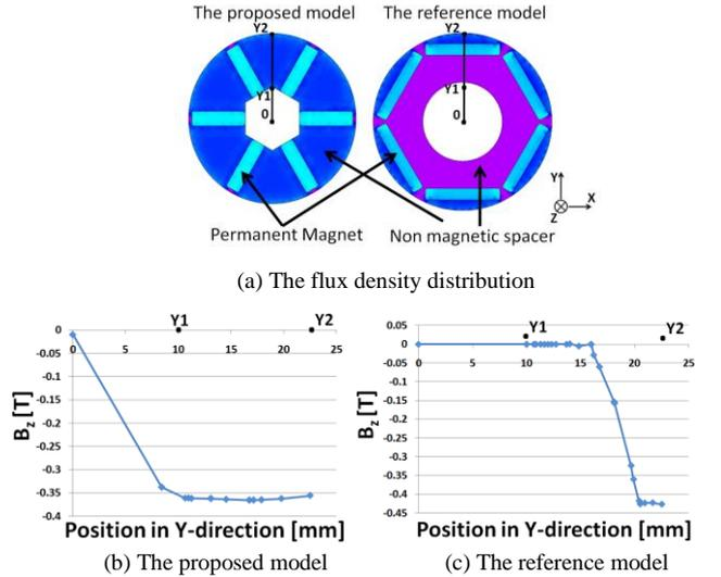
Figure 7: The flux density in non-magnetic material spacer.
