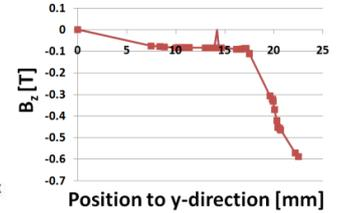
(a) The flux density distribution in non-magnetic material spacer
