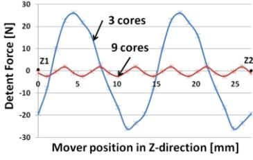
Figure 4: Detent force of the proposed model.
