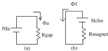
Fig. 5. Motor magnetic circuit model. (a) Armature magnetic circuit. (b) Field magnetic circuit.
