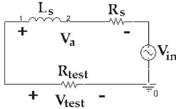
Fig. 12. Stationary ac input armature impedance test circuit.
