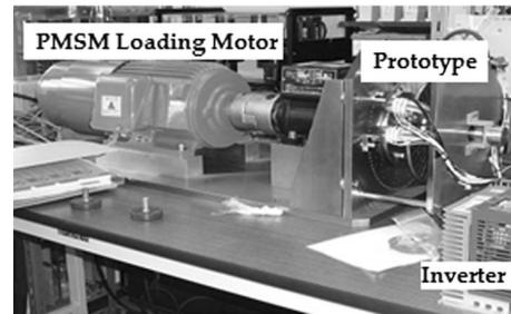
Fig. 9. Prototype test bench.
