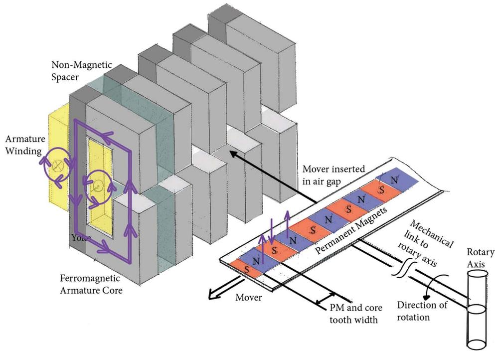
Fig. 3. Flux path through the C-core and rotor.
