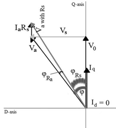
Fig. 6. Phasor diagram for a symmetrical three-phase machine.
