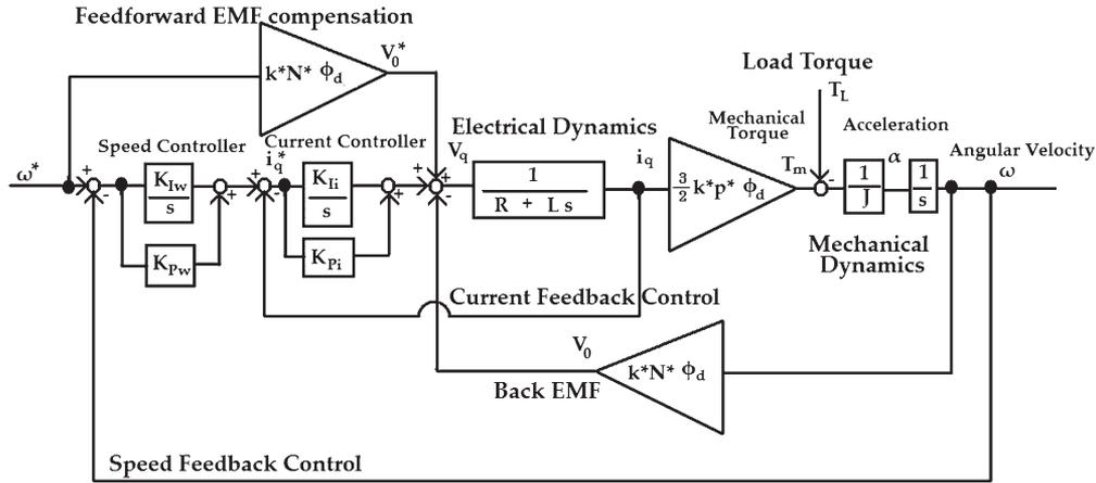
Fig. 16. Cascaded PI speed controller and  $Q$ -axis current controller.
