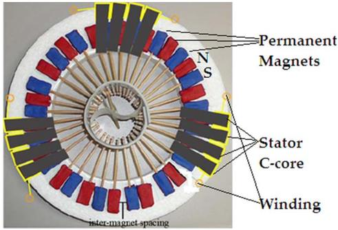
Fig. 7. Illustration of a rotary disk motor design concept.
