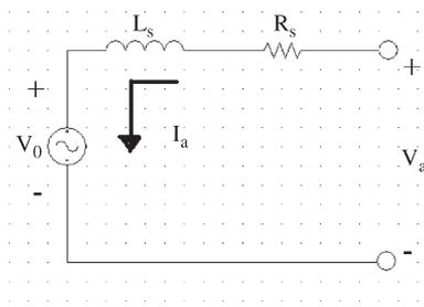
Fig. 4. Per phase equivalent circuit model.
