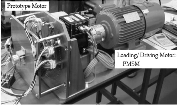
Fig. 6: A Full Version of the Prototype Motor Model<sup>[7]</sup>
