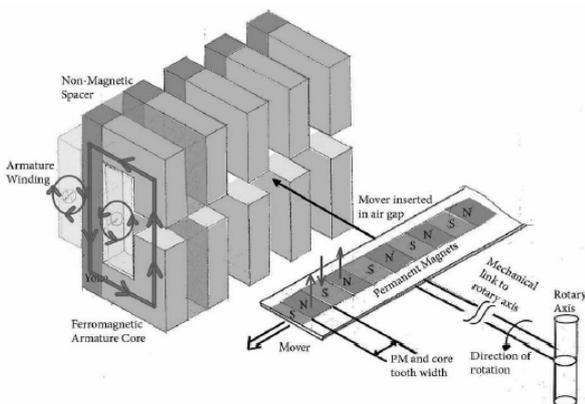
Fig. 3: Flux Path through C-Core and Rotor<sup>[7]</sup>
