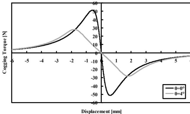
Fig. 19: Cogging Torque per a Pole Depending on Skew Angle
