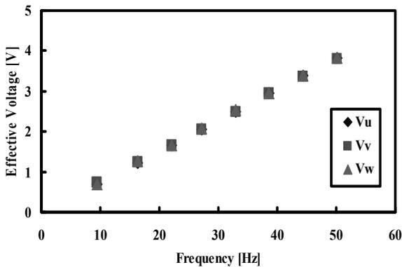
Fig. 13: Effective Voltage in the Open Circuit Test
