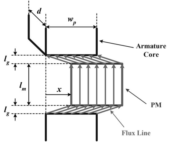
Fig. 17: The Simplified Flux Line in the Air Gap
