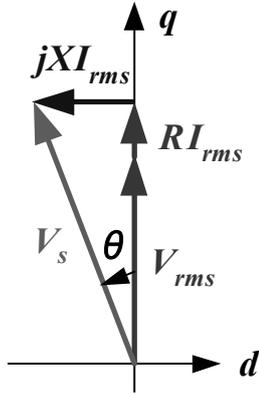
Fig. 16: Phasor Diagram of Voltages and Currents ( $I_d = 0$ )
