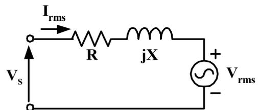
Fig. 15: One Phase Equivalent Circuit
