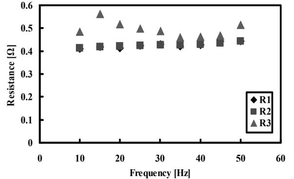
Fig. 11: AC Resistance Measurement
