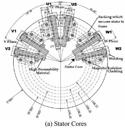
(a) Stator Cores
