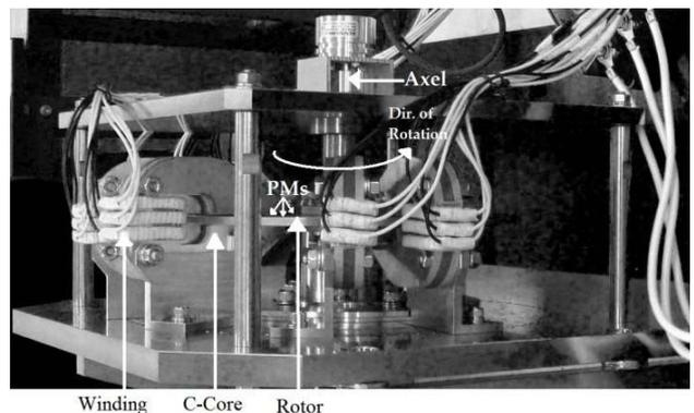
Fig. 5: Detailed Parts of the Prototype Motor<sup>[7]</sup>
