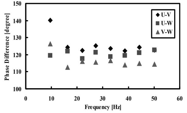
Fig. 14: Phase Difference in the Open Circuit Test
