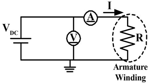
Fig. 7: DC-Voltage Drop Test Circuit
