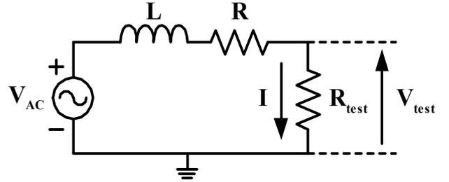
Fig. 9: The Test Circuit for Measuring Self-Inductance
