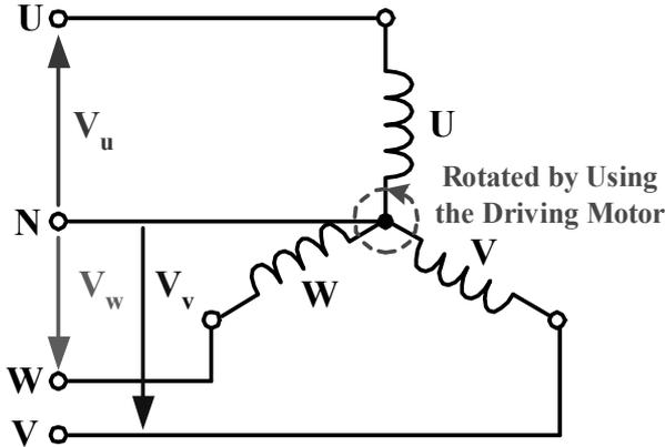
Fig. 12: The Test Circuit for Measuring Self-Induced Voltage
