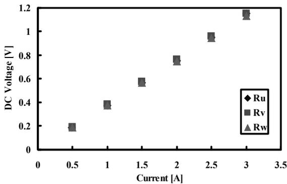
Fig. 8: Armature Resistance Measurement
