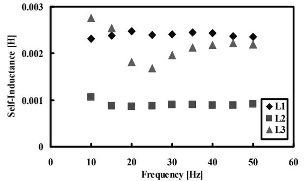
Fig. 10: Self-Inductance Measurement
