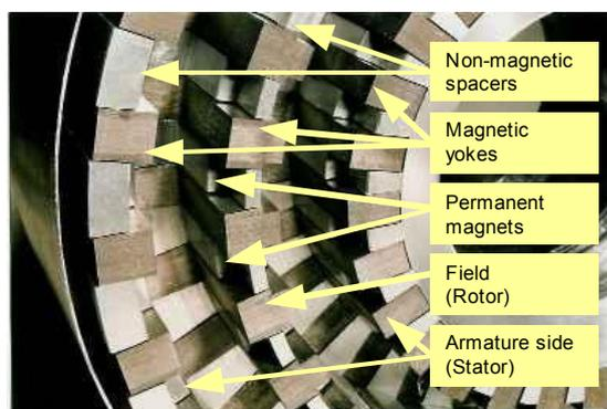
Fig. 1 The first prototype transversal flux-motor tested at the Technical University in Braunschweig in 1989.
