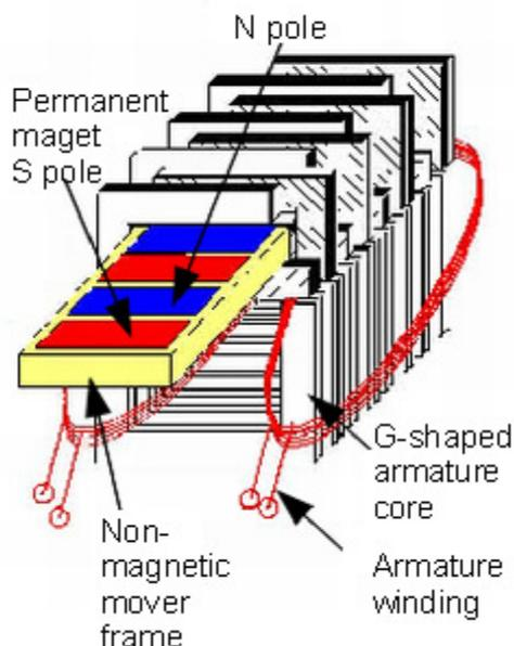
Fig. 2 Tunnel actuator proposed by Kim, Hitachi Ltd. Corp.
