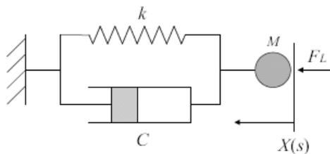
Fig. 7 A mechanical dynamic system to be emulated through a force-control-type stiffness/viscosity control.
