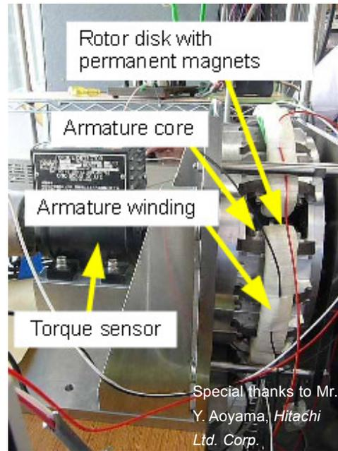
Fig. 5 The second prototype of the disk-rotor transversal flux synchronous machine at the University of Tokyo.
