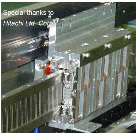
Fig. 3 An early prototype of the Tunnel Actuator developed for industrial machine tools.
