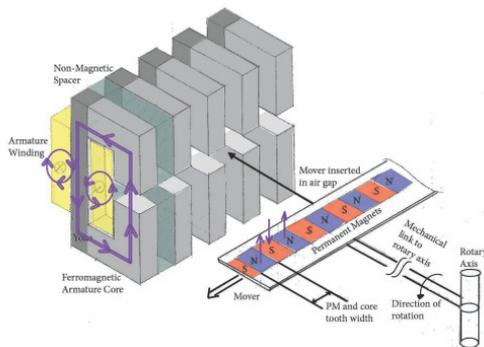
Fig. 3 Fundamental diagram of a rotary transversal flux motor extended from tunnel actuators being developed by Koseki.
