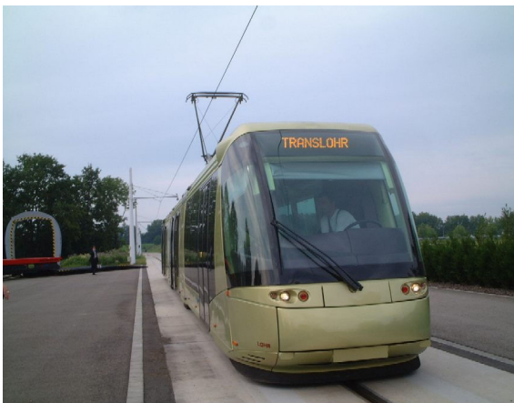
Fig. 8 Translohr on a road guided by a single rail.
