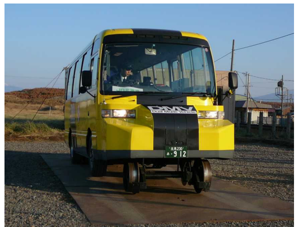
Fig. 9 Dual Mode Vehicle as a combination of rail-guided public transport and a bus developed by JR-Hokkaido.
