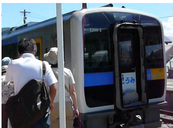
Fig. 10 Diesel hybrid train Kiha-E200 developed by JR-East and applied to Koumi-Line.
