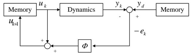
Fig. 3. Block diagram of P-Type learning control[4].
