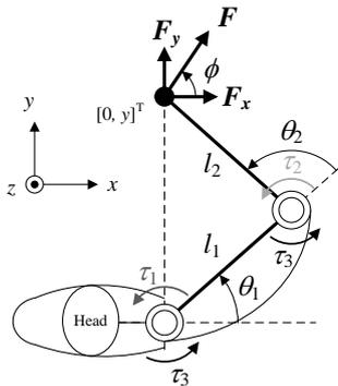
Fig. 2. Fundamental 2-link arm model[2].
