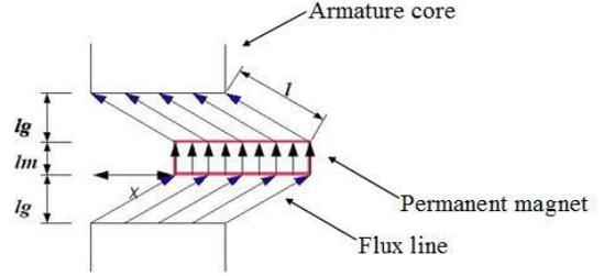
Fig. 7. Flux line in the air gap
