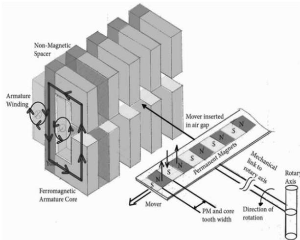
Fig. 3. Flux path through C-core and rotor<sup>[7]</sup>
