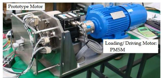
Fig. 6. A full version of the prototype motor model<sup>[7]</sup>
