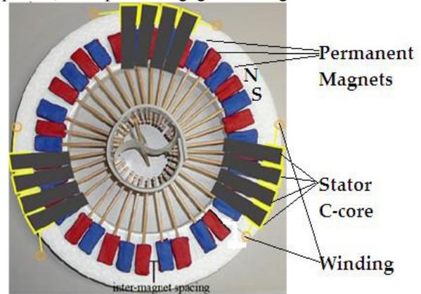
Fig. 4. The illustration of the prototype motor model<sup>[7]</sup>
