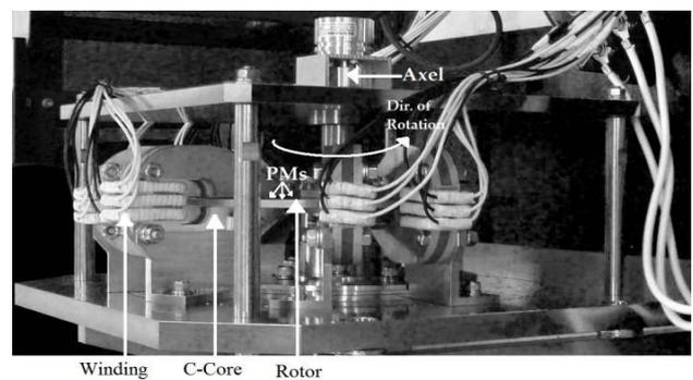
Fig. 5. Detailed parts of the prototype motor<sup>[7]</sup>
