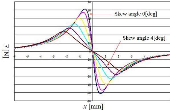
Fig. 8. Cogging torque per a pole depending on skew angle
