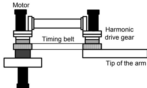
Fig. 9. Improvement model for two links rotating system.
