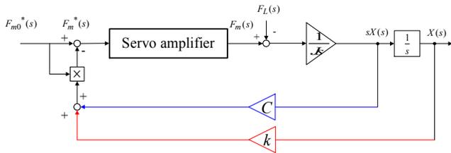
Fig. 4. Thrust control type mechanical impedance control system.
