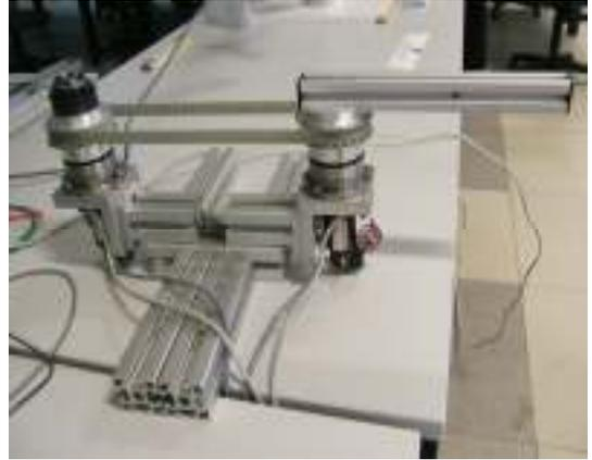
Fig. 3. Experimental machine which has two rotary motors as role of an elbow and a bi-articular muscle.
