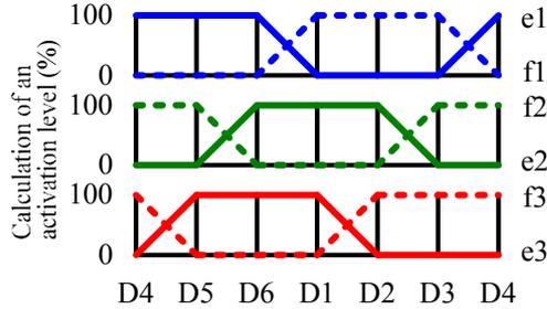
Fig. 2. Theoretically calculated activation level of each muscle can be applied on torque pattern of each actuator respectively [1].
