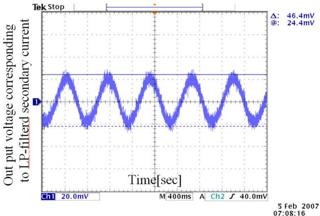
Figure 11: Normal output at 1079.0Hz (20th harmonic)
