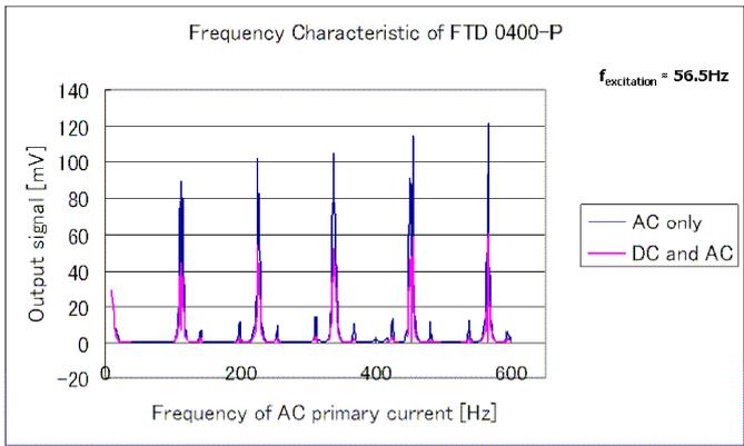
Figure 4: Frequency characteristics of FTD 0400-P
