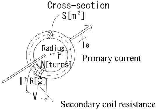
Figure 1: Diagram of a single core-type fluxgate direct current sensor
