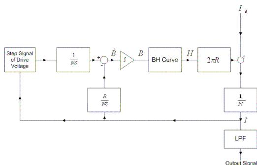
Figure 2: Block diagram of the fluxgate sensor operation
