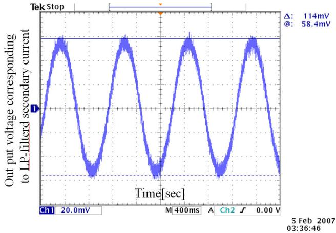
Figure 9: Normal output at 109.5Hz(2nd harmonic)
