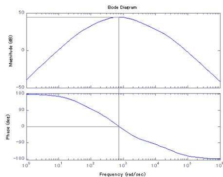
Figure 7: Bode diagram of functional block responsible for phase shift in AC signal
