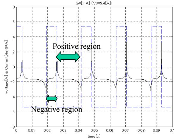
Figure 3: Voltage steps and current response in secondary winding (Primary current = 2[A])
