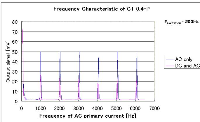
Figure 5: Frequency characteristics of Current Transducer 0.4-P
