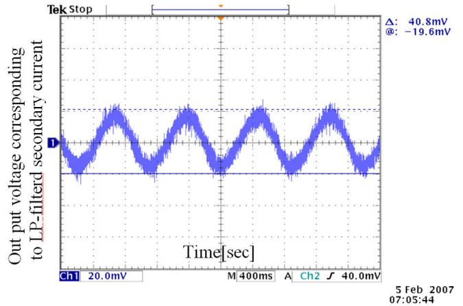
Figure 12: With compensation at 1079.0Hz (20th harmonic)
