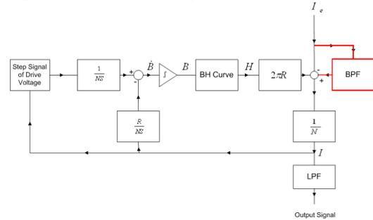
Figure 6: Block diagram with an Active AC-component compensation
