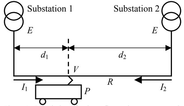
Figure 2. Calculation of voltage fluctuation at pantograph
