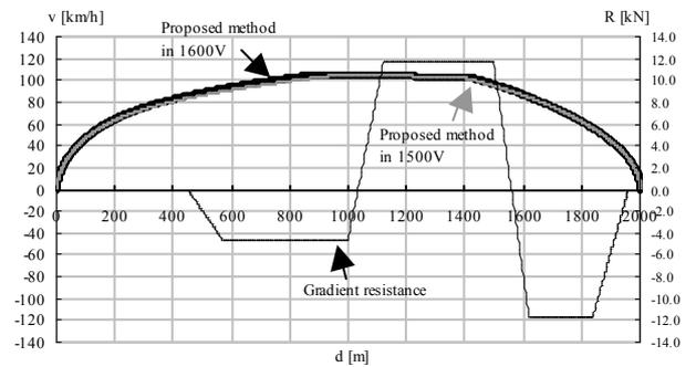
Figure 8. Comparison of run curve at a station interval in different output voltages at substations
