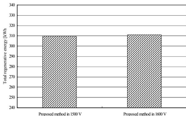
Figure 10. Comparison of regenerated energy in different output voltages at substations
