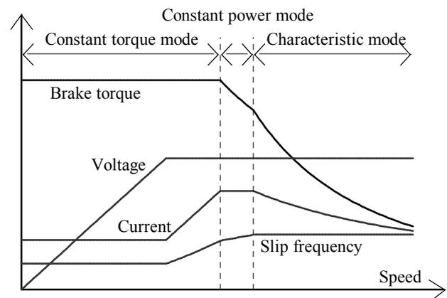
Figure 1. Speed characteristics of an electric train driven by induction motor
