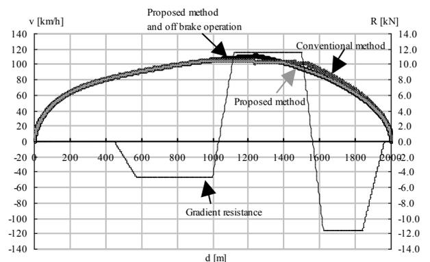
Figure 3. Comparison of run curve at a station interval
