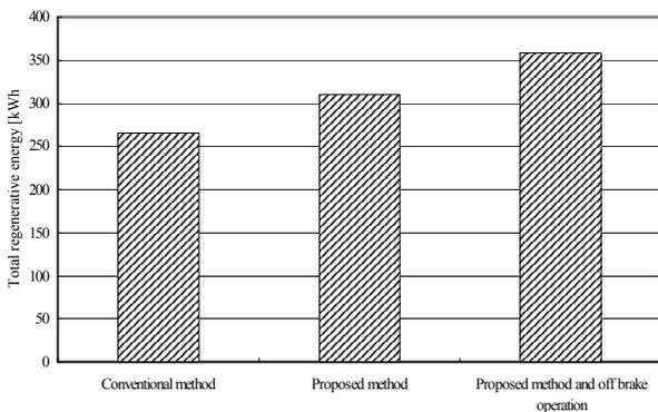
Figure 5. Comparison of regenerated energy
