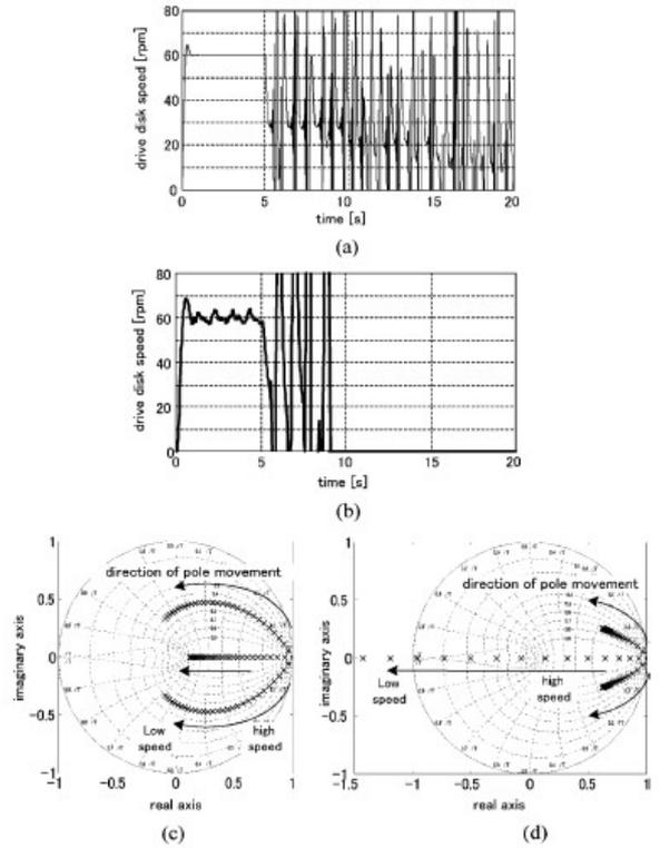
Fig. 4 (a) Simulation and (b) experimental results of the conventional pole assignment. (c) Movement of the poles in design. (d) Actual movement of the poles.
