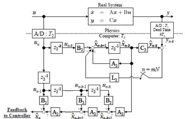
Fig. 7. Block diagram for estimating state variables of a plant with dead time in output signal path.
