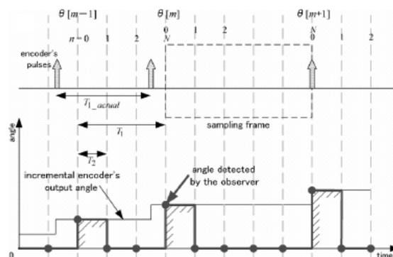
Fig. 1. Timing diagram of the dual-sampling-rate observer when the period between two consecutive pulse is larger.
