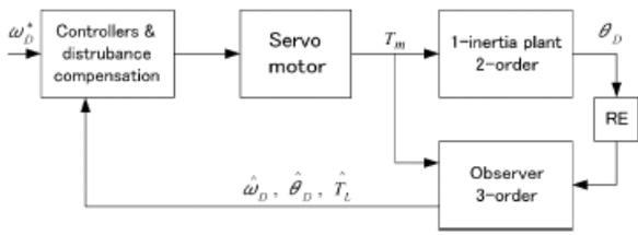
Fig. 6. Block diagram for verification of the pole assignment method.
