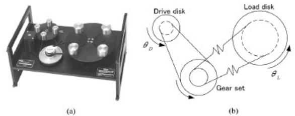
Fig. 5 (a) Experimental apparatus. (b) Free body diagram.
