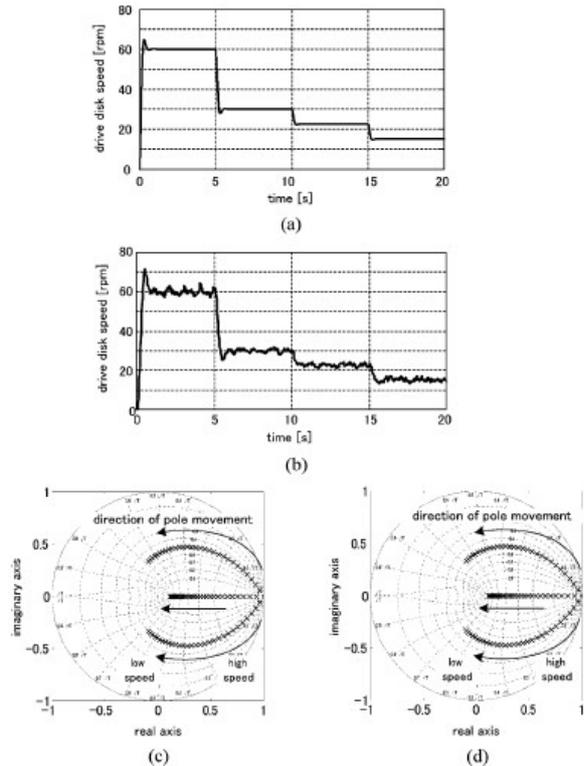
Fig. 3 (a) Simulation and (b) experimental results of the proposed pole assignment. (c) Movement of the poles in design. (d) Actual movement of the poles.
