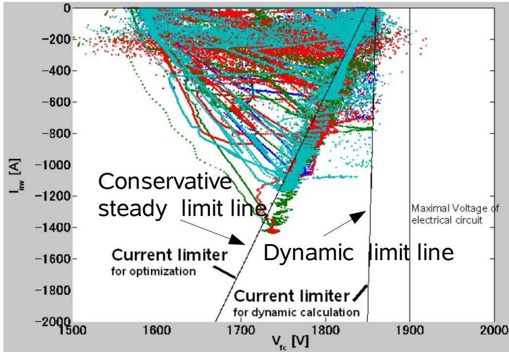
Fig. 8 Limit lines and calculated  $V$ - $I$  loci when the train 4 is an old type.
