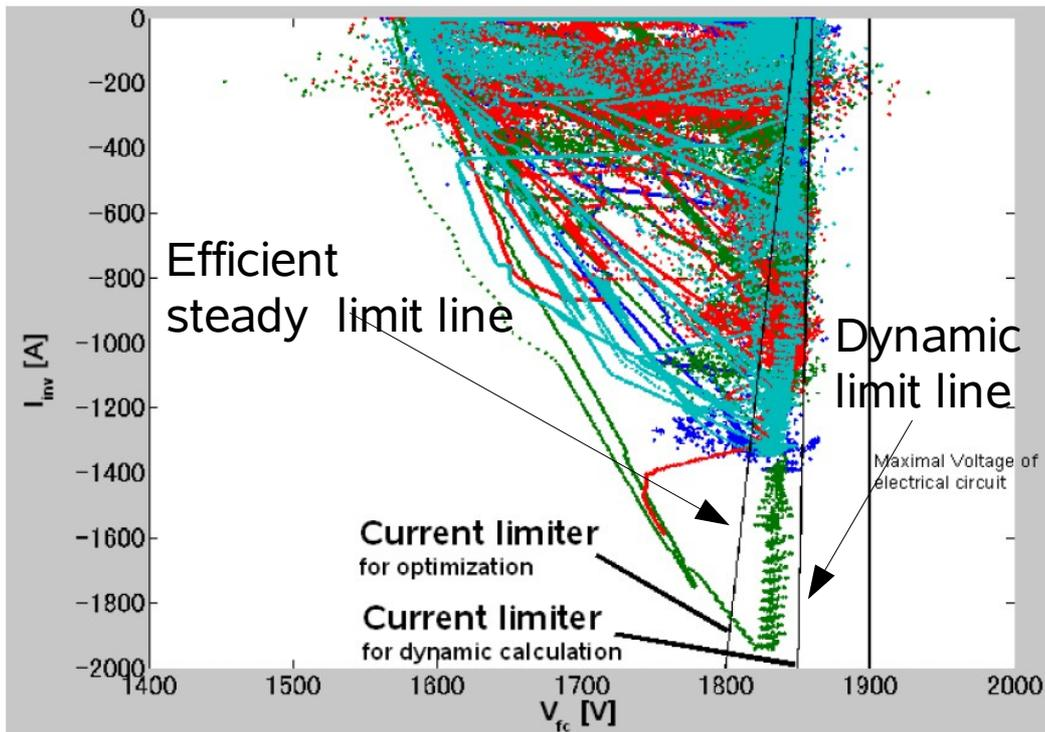
Fig. 10 Limit lines and calculated  $V$ - $I$  loci when the train 4 is a new type.
