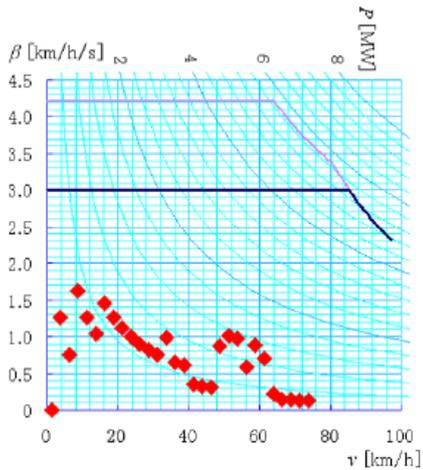
Fig. 4 Summary of measured electric braking operation.
