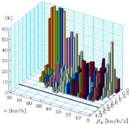
Fig. 3 Normalized frequency of measured electric brake-operating points.
