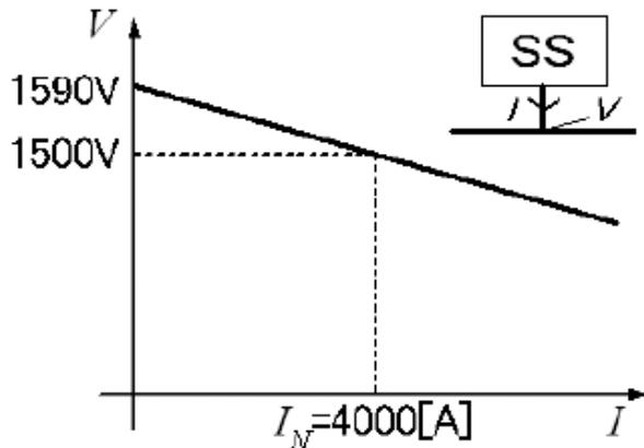
Fig. 9  $V$ - $I$  characteristics of a substation.
