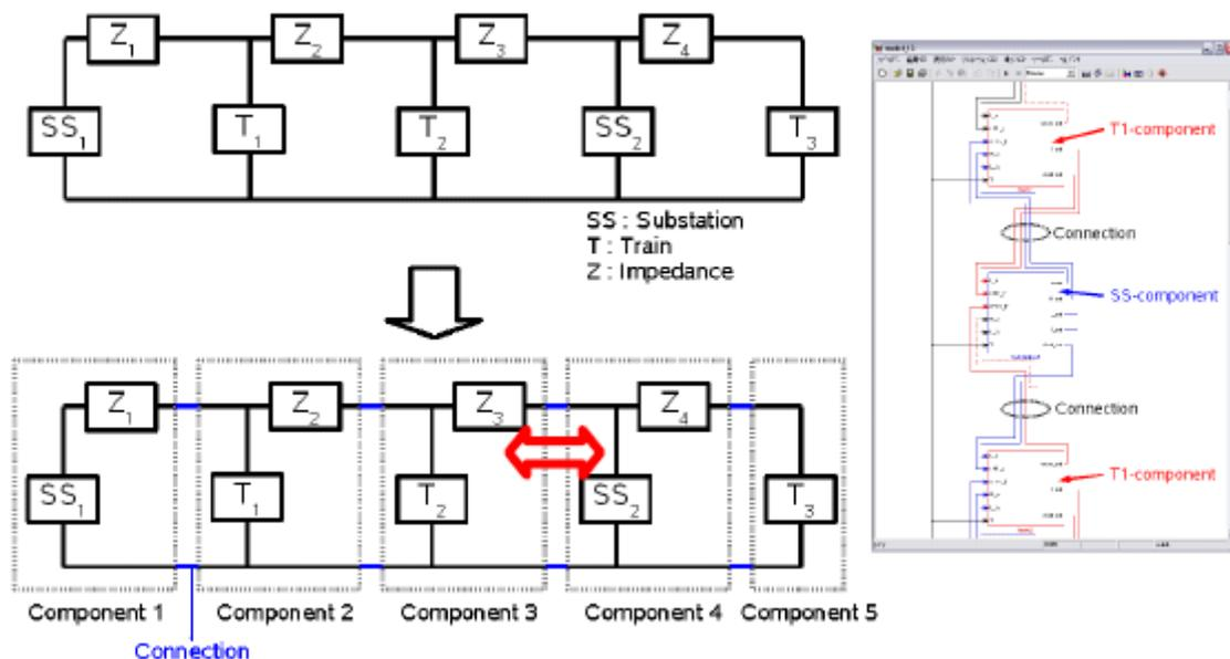
Fig. 1. Fundamental block for dividing a DC-electrification circuit to functional blocks for a transient simulator using MATLAB and SIMULINK.
