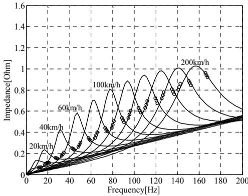
Fig. 6. Frequency characteristics of absolute value of impedance  $|Z|$
