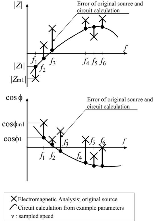
Fig. 4. Curve-fitting scheme of identification of circuit parameters under constant speed
