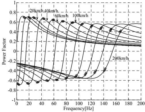
Fig. 7. Frequency characteristics of power factor  $\cos\phi$
