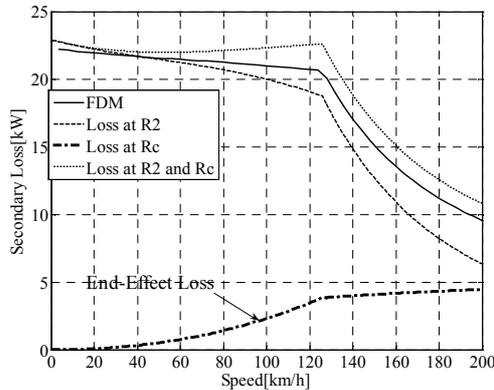
Fig. 15. Characteristics of secondary copper loss and the end-effect loss
