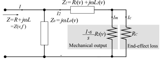
Fig. 11. Per-phase equivalent circuit of LIM including end-effect loss
