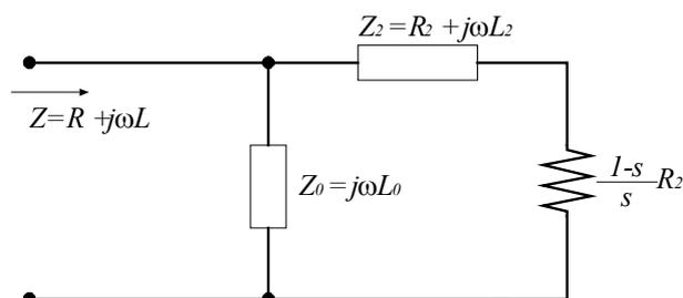
Fig. 1. Per-phase equivalent circuit of conventional induction motor
