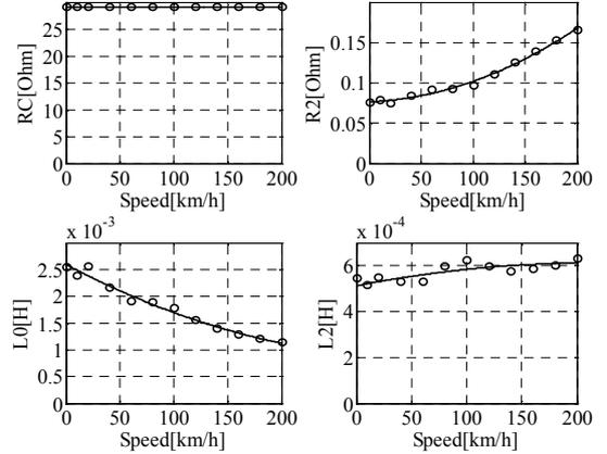
Fig. 12. Characteristics of circuit parameters depending on speed with the end-effect loss  $R_c$
