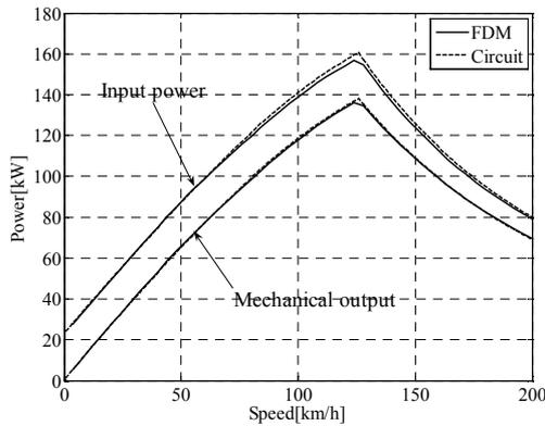
Fig. 14. Characteristics of input power and mechanical output
