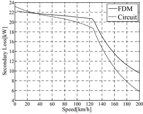
Fig. 11. Characteristics of secondary copper loss
