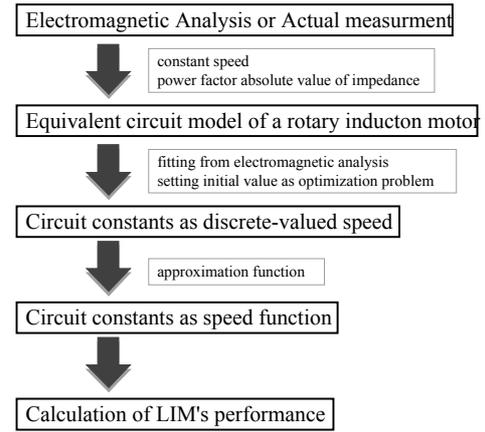
Fig. 3. New identification method of equivalent circuit for a LIM
