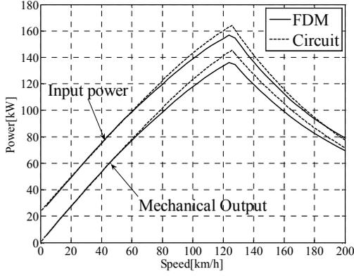
Fig. 10. Characteristics of input power and mechanical output
