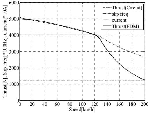
Fig. 13. Characteristics of traction force including end-effect loss
