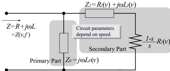
Fig. 2. Per-phase equivalent circuit extended for a LIM
