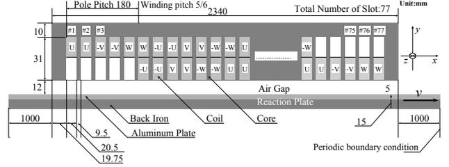
Fig. 5. Analytical model of a LIM based on HSST-200 vehicle
