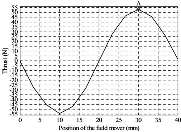
Fig. 7. Change of thrust with the movement of the field mover by two-dimensional FEM.
