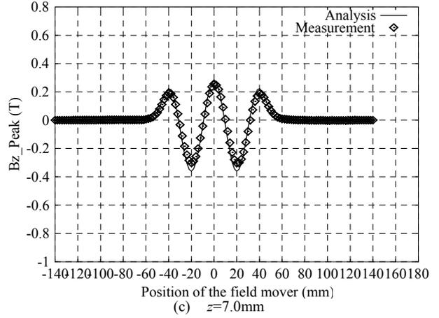
Fig. 6. Comparison of analysis and measurement about the flux density distribution of the field mover.
