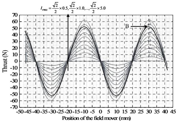
Fig. 8. Change of thrust with the movement of the mover on the condition of a constant current by measurement.
