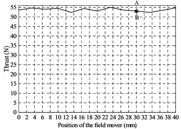
Fig. 9. Change of thrust with the movement of the mover on the condition of a phase difference angle  $=\pi/2$  by two-dimensional FEM.
