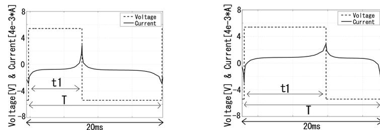
Figure 5: Input Voltage and Output Current ( $I_e = 1[A]$ )
