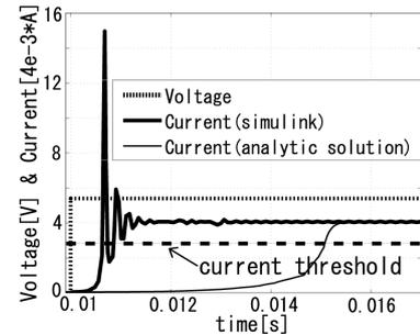
Figure 3: Step response of current
