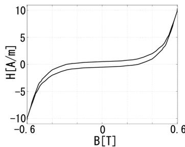
Figure 2: HB-hysteresis curve approximated by broken lines
