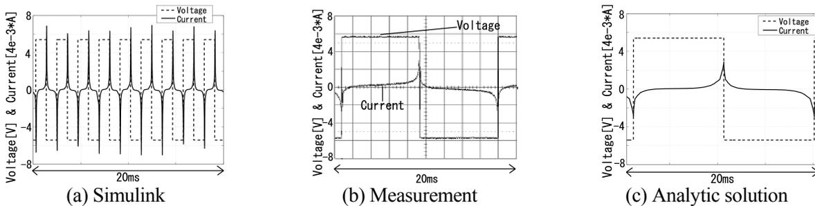
Figure 4: Input Voltage and Output Current ( $I_e=0[A]$ )
