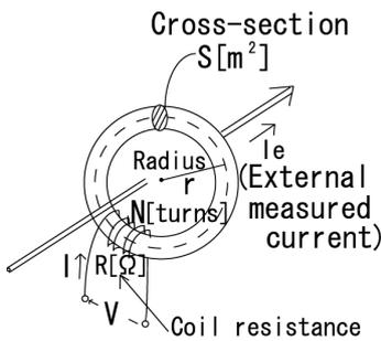
Figure 1: Fundamental magnetic circuit model for a flux-gate sensor
