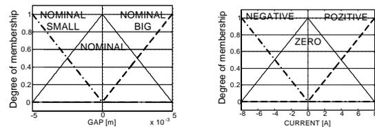
Fig. 4. Fuzzy membership functions of the gap clearance and coil currents.
