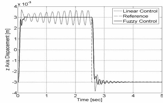
Fig. 9.  $z$  axis time response for reference change without disturbance feed-forwarding.
