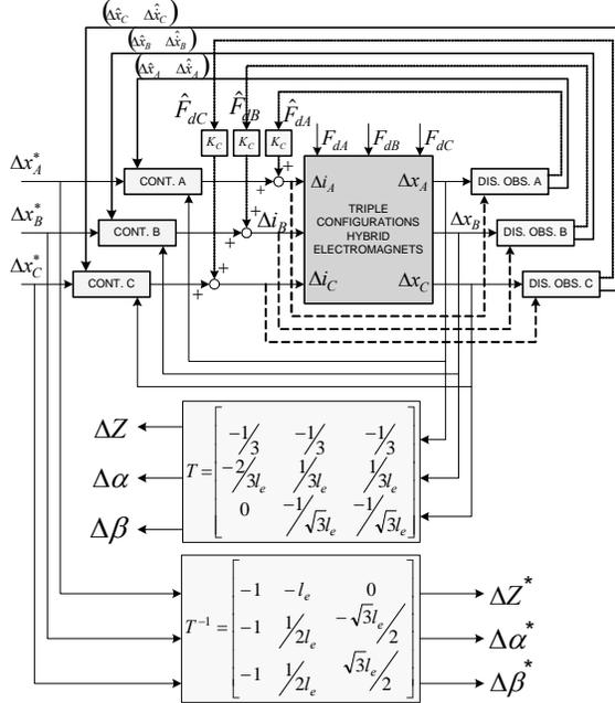
Fig. 6. Block diagram of the linear control system.
