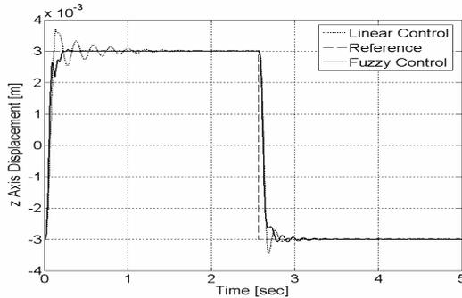
Fig. 11.  $z$  axis time response for reference change with disturbance feed-forwarding.
