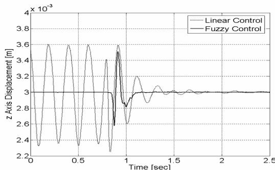
Fig. 13.  $z$  axis time response for  $1.2 [kg]$  pay-load disturbance acting @  $0.874 [sec]$  without disturbance feed-forwarding.
