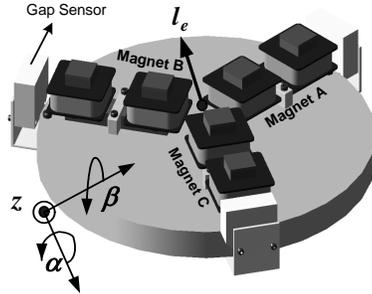
Fig. 2. Triple configuration of hybrid electromagnets on a plane.
