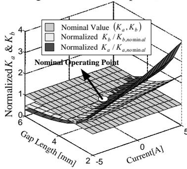
Fig. 3. Normalized variations of magnet stiffness parameters,  $K_a$  &  $K_b$ , according to change of operating point.
