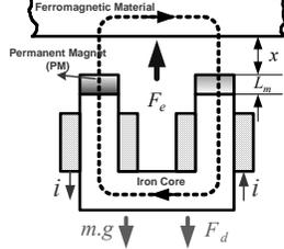
Fig. 1. Essential structure of a U-shaped hybrid electromagnet for one-dimensional motion case.
