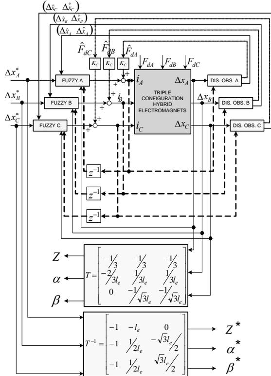
Fig. 7. Block diagram of the proposed fuzzy control system.
