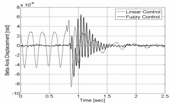
Fig. 14.  $\beta$  axis time response for  $1.2 [kg]$  pay-load disturbance acting @  $0.874 [sec]$  without disturbance feed-forwarding.
