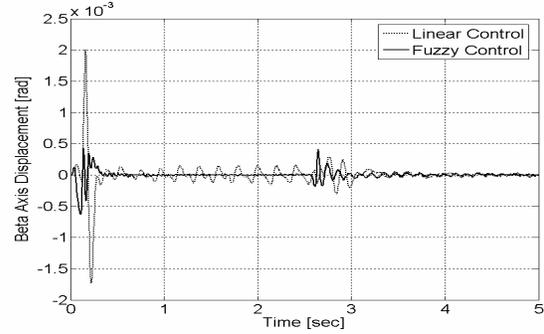
Fig. 10.  $\beta$  axis time response for reference change without disturbance feed-forwarding.
