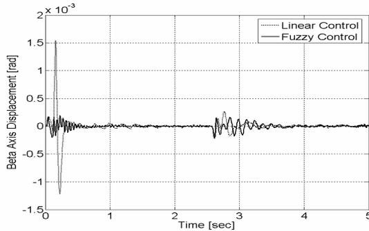
Fig. 12.  $\beta$  axis time response for reference change with disturbance feed-forwarding.
