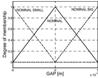
Fig. 2. Membership functions for gap clearance.
