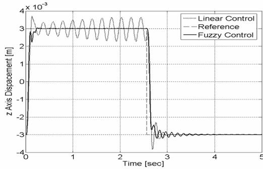
Fig. 7.  $z$  axis time response for reference change without disturbance feed-forwarding.
