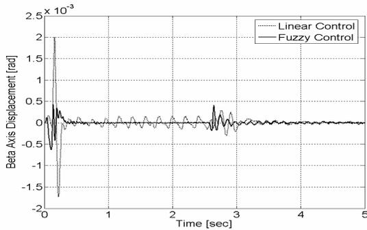
Fig. 8.  $\beta$  axis time response for reference change without disturbance feed-forwarding.
