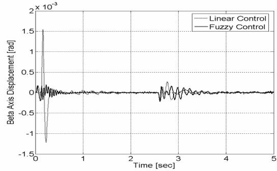
Fig. 10.  $\beta$  axis time response for reference change with disturbance feed-forwarding.
