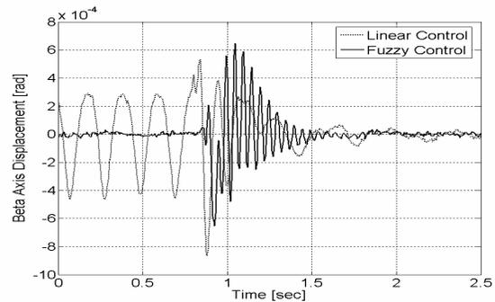
Fig. 12.  $\beta$  axis time response for  $1.2 [kg]$  pay-load disturbance acting @  $0.874 [sec]$  without disturbance feed-forwarding.
