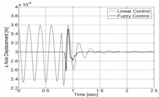
Fig. 11.  $\beta$  axis time response for  $1.2 [kg]$  pay-load disturbance acting @  $0.874 [sec]$  without disturbance feed-forwarding.
