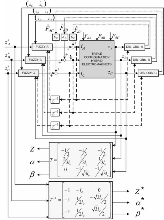
Fig. 6. Fuzzy control systems block diagram.
