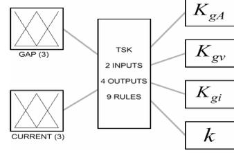
Fig. 4. Fuzzy controller block diagram for magnet A.
