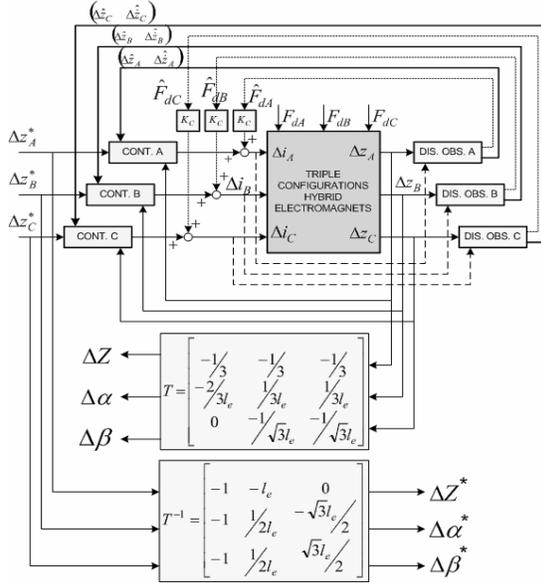
Fig. 5. Linear control system block diagram.
