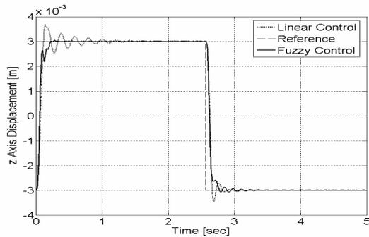
Fig. 9.  $z$  axis time response for reference change with disturbance feed-forwarding.
