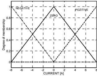
Fig. 3. Membership functions for current.
