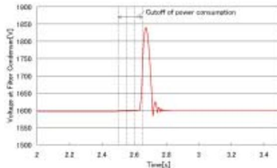
Figure 12: Voltage at the filter capacitor (3)
