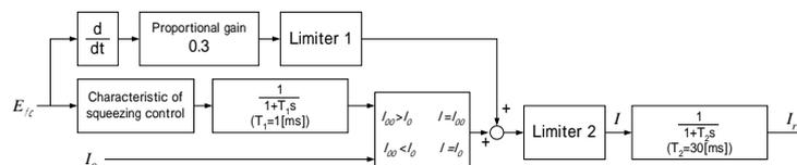
Figure 11: Operation logic for squeezing control (2)
