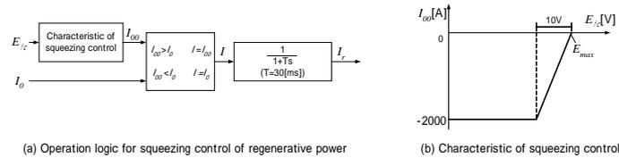
Figure 6: Operation logic for squeezing control (1)
