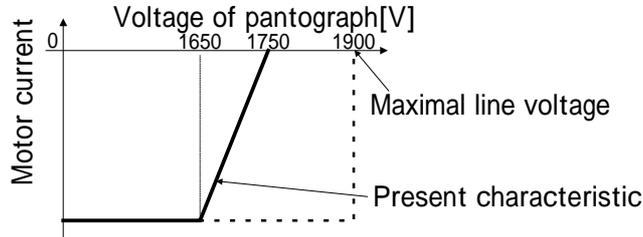
Figure 2: Typical characteristic of squeezing control
