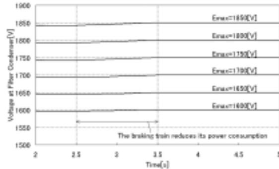
Figure 7: Voltage at the filter capacitor (1)
