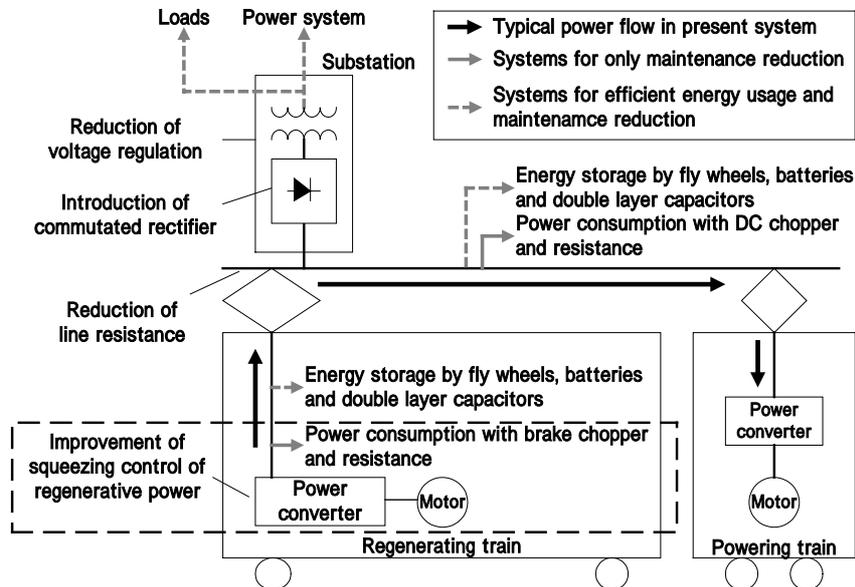
Figure 1: Typical power flow on braking
