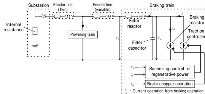
Figure 3: Electrical circuit for examination
