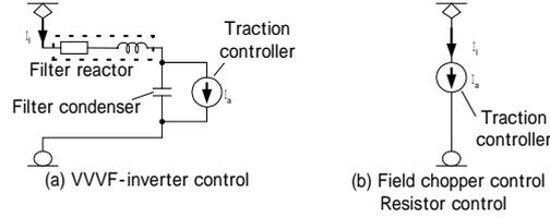
Figure 4: Equivalent circuits of powering train
