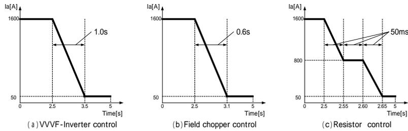
Figure 5: Characteristics at cutoff of power consumption
