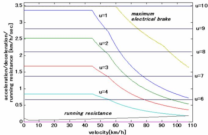
Figure 4: Acceleration/deceleration performance and running resistance.
