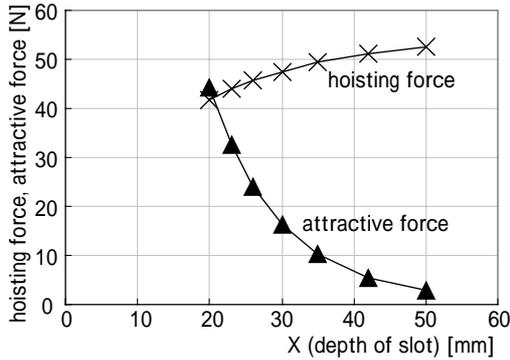
Fig. 5 Hoisting Force and Attractive Force of the LSM
