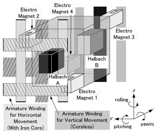
Fig. 1 Structure of Proposed Vertical Transport System
