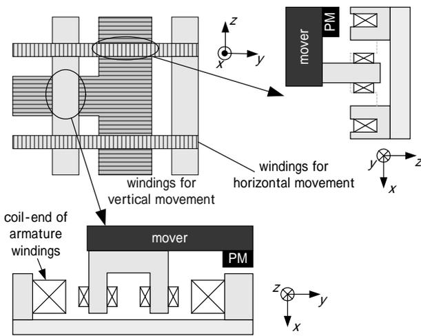
Fig. 2 Structure at Shunting Place
