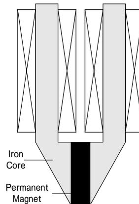
Fig. 6 U-shaped Electromagnet for Levitation Control
