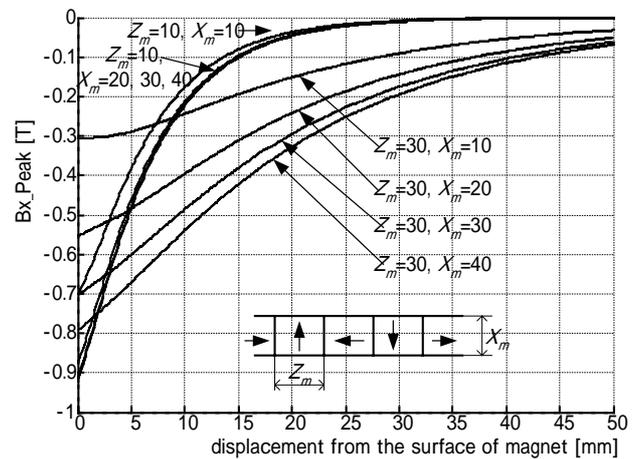
Fig. 4 Influence of the magnet size to Magnetic Flux
