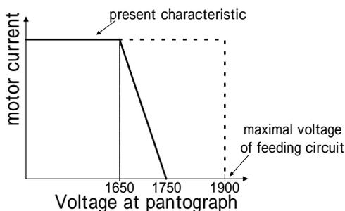
Fig1 Characteristic of Squeezing Control
