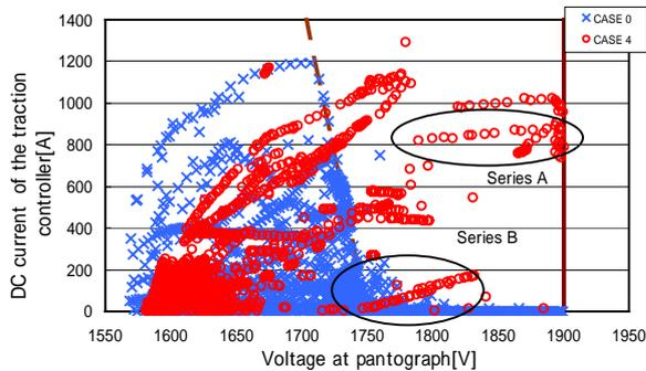
Fig.4 The Relation of the Voltage at Pantographs and the DC Current of Traction Controller
