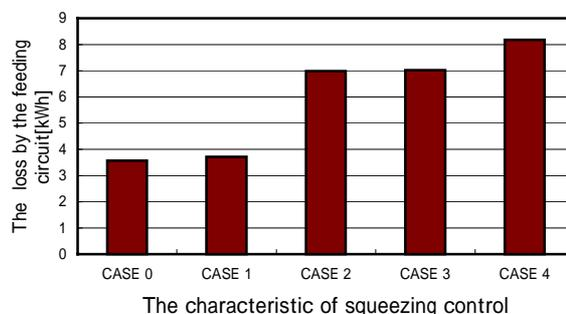
Fig.8 The Loss by Feeding Resistance
