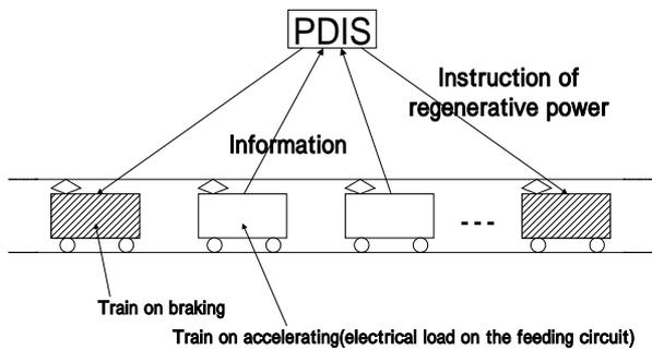
Fig.2 The Concept of PDIS
