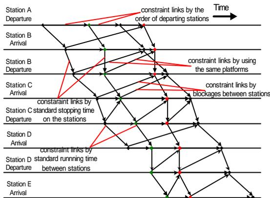
Fig. 1 The graph structure represents train operation
