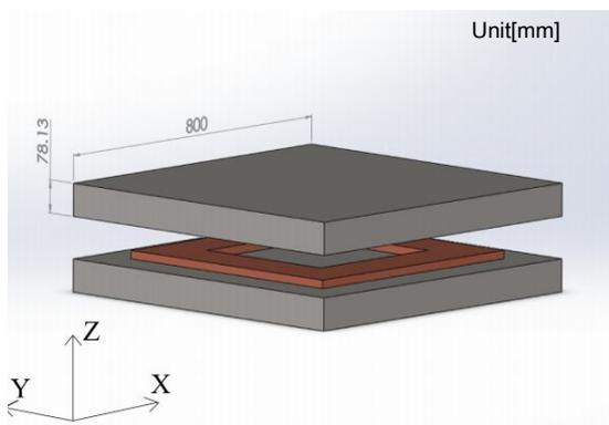
Fig.2 Structure and size of the transformer using square cores
