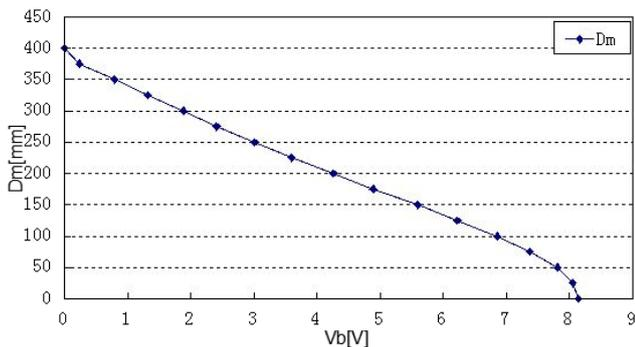
Fig.11 Distance-voltage characteristic
