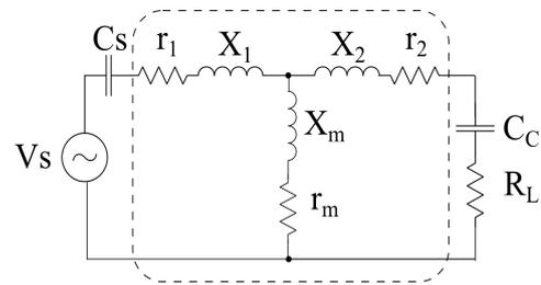
Fig.3 Equivalent circuit of the transformer
