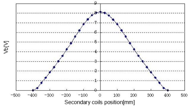
Fig. 9  $V_b$  when secondary coils are at each position
