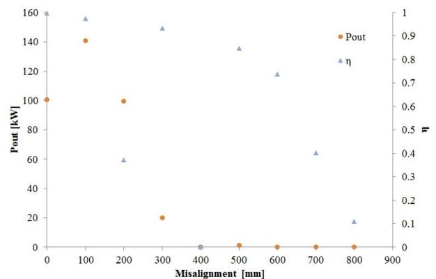
Fig.4 Power transfer performance of transformer using square cores
