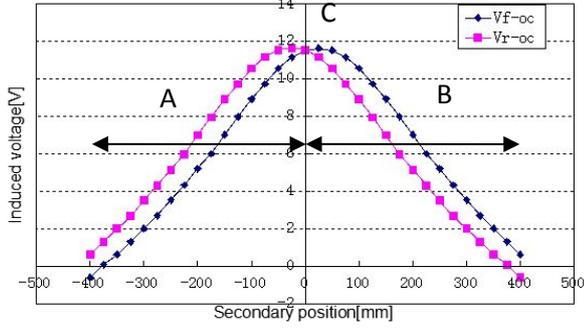
Fig.8 Voltage induced in secondary coils
