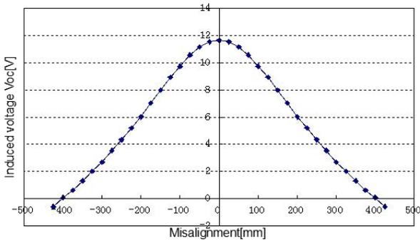
Fig.6 Voltage induced in secondary coil
