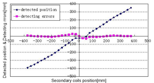
Fig.13 Detected position of secondary coils in case of deviation
