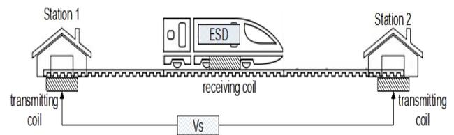
Fig.1 Configuration of static wireless charging system for railway
