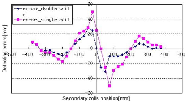
Fig.14 Errors of two distance detection methods
