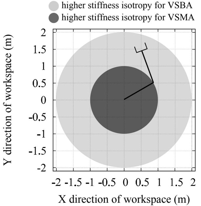
Fig. 5. Regions of the workspace of the two-link robot arm where the VSMA and VSBA are advantageous in terms of stiffness isotropy
