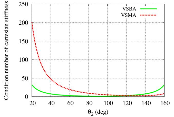
Fig. 4. Condition numbers of Cartesian stiffness in respect to  $\theta_2$
