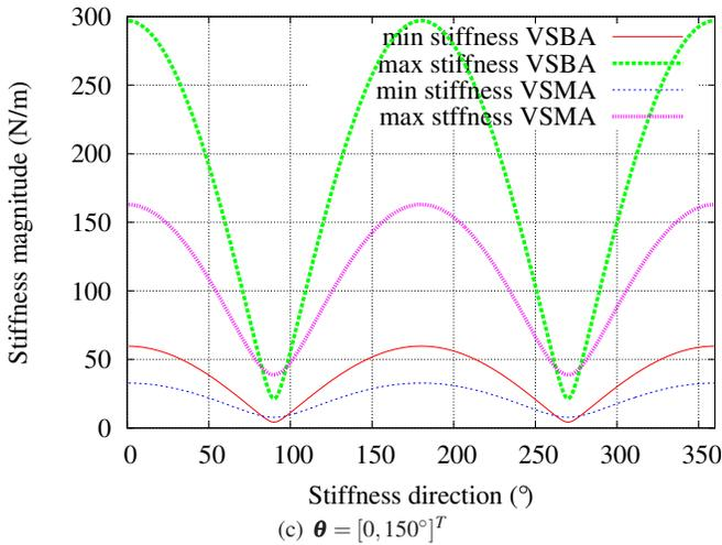
Fig. 3. Minimum and maximum end effector Cartesian stiffness
