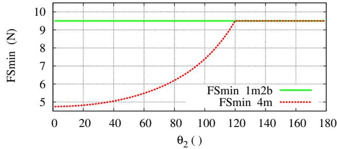
Fig. 3.  $|FSmin|$  for  $4m$  and  $1m2b$  structures in respect to  $\theta_2$ .  $\theta = [0, (1 - 179)^\circ]^T$
