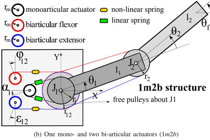
Fig. 1. Two-link intrinsically compliant manipulators: conventional and proposed structures
