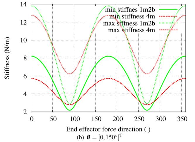
Fig. 4. Minimum and maximum end effector Cartesian stiffness ( $|F^{out}| = 0$ )
