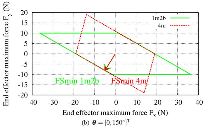
Fig. 2. Maximum output force space and resulting minimum force ( $FSmin$ ) for both actuation structure
