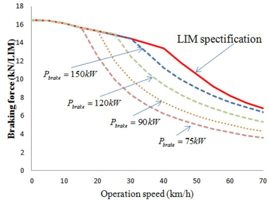
Fig.2. Different power limited brake
