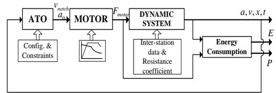
Fig.1. Block diagram of the modularized model simulator
