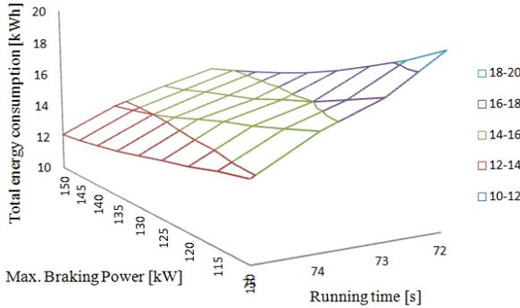
Fig.4. Total energy consumption and maximal braking power in running time relations
