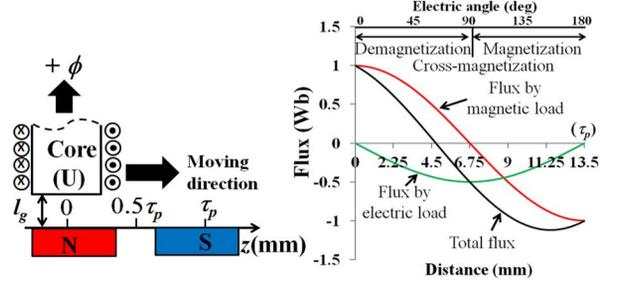
Fig. 4. Flux distribution in the armature core due to armature reaction. (The positive value on the left side represents the direction in which the flux flows into the iron core).
