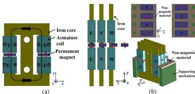
Fig. 1. The basic configuration of the three-phase unit. (a) Armature and field units. (b) Configuration along the moving direction. (In (a), black arrows denote flux flow under a no-load condition. In (b),  $-U$ ,  $-V$ , and  $-W$  are present components shifted by 180 degrees from  $U$ ,  $V$ , and  $W$ ).
