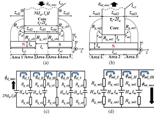
Fig. 6. Magnetic circuit models for flux calculation by electric and magnetic loads. (a) Model at  $z = 0.5 \tau_p$ . (b) Model at  $z = 0$ . (c) Equivalent magnetic circuit at  $z = 0.5 \tau_p$ . (d) Equivalent magnetic circuit at  $z = 0$ . (Only a half model is illustrated because of the symmetric structure).
