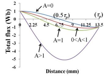
Fig. 5. Total flux distribution by the flux ratio  $A$ .
