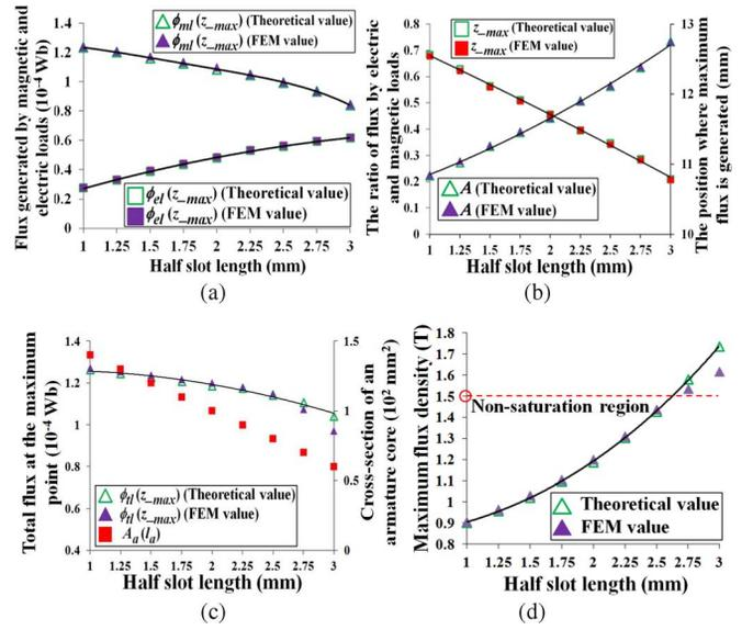
Fig. 7. Theoretical and 3-D FEM results. (a)  $\phi_{ml\_max}$  and  $\phi_{el\_max}$ . (b)  $A$  and  $z_{-max}$ . (c)  $\phi_{t1}(z_{-max})$  and  $A_a(l_a)$ . (d)  $B_{max}$ .
