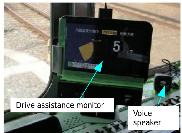
Fig. 8 Driver interface of the onboard drive assistance system
