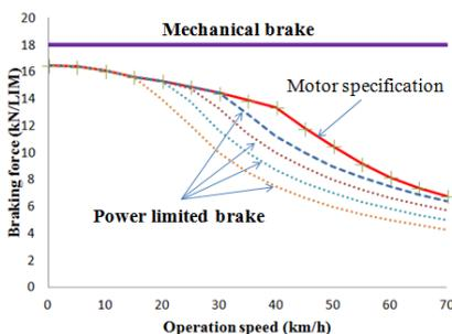
Fig. 2. Different braking modes
