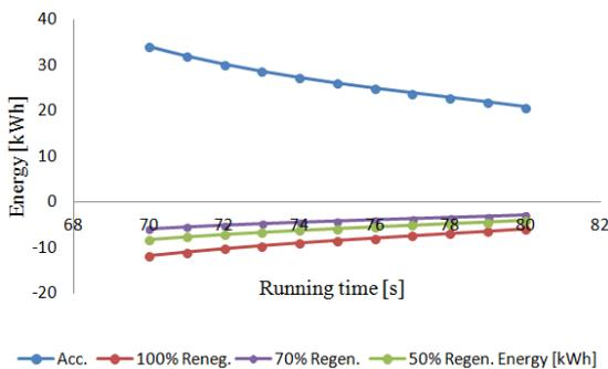
Fig. 6. Acceleration and regenerative energy
