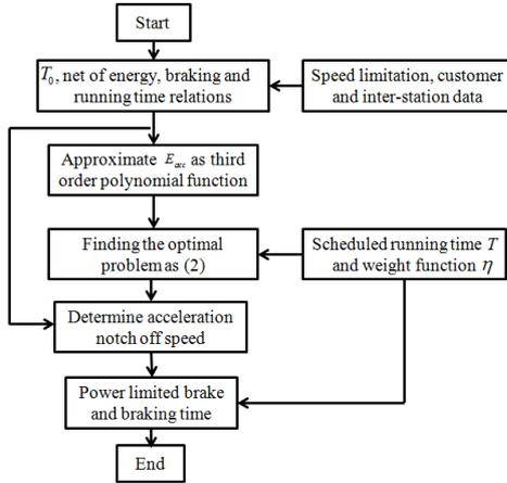
Fig. 9. Flow chart of running curve design
