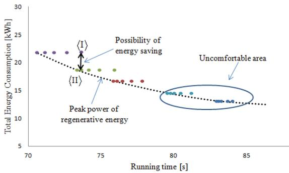
Fig. 4. Relation between the net of energy consumption and the running time
