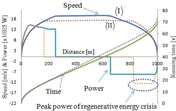
Fig. 5. Comparison between conventional <I> and lowest energy consumption <II> running curve
