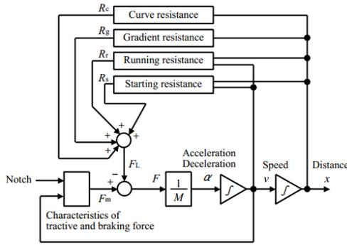
Fig. 4. Numerical calculation of a train motion [3]
