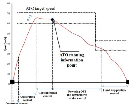
Fig. 3. Speed profile of a possible lower notch-off speed and power limited brake pattern
