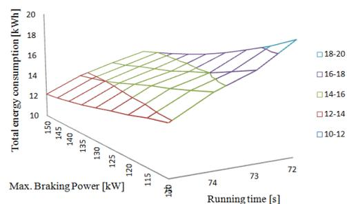
Fig. 2. Braking power and total energy consumption in running time relations
