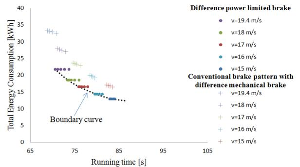
Fig. 5. Net of energy consumption and running time of a train in a substation
