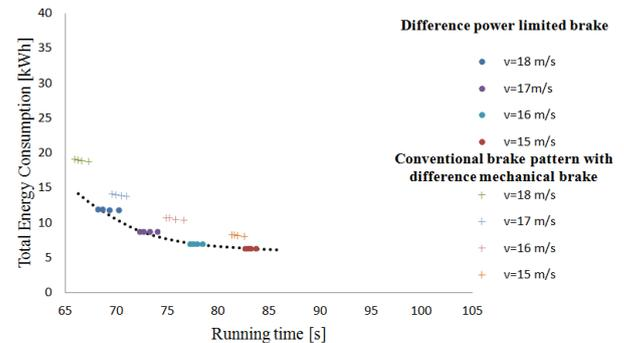
(b) Downward slope with 8% gradient
