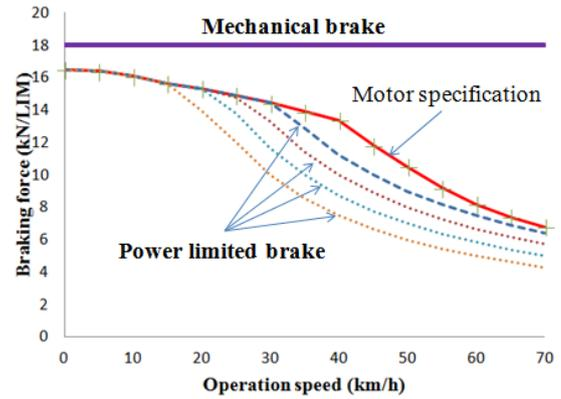
Fig. 2. Difference braking modes
